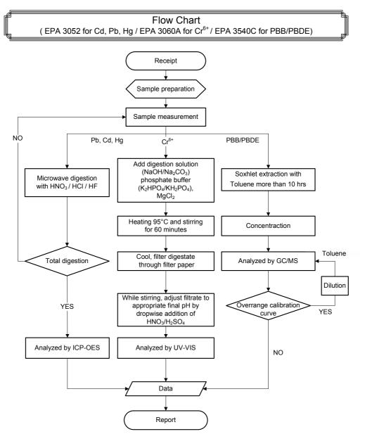
\*\* Remarks : The samples were dissolved totally by pre-conditioning method according to above flow chart.
